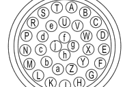
ME connector (32 pin) Glenair IPT 02 A 18-32 P F6 front view
